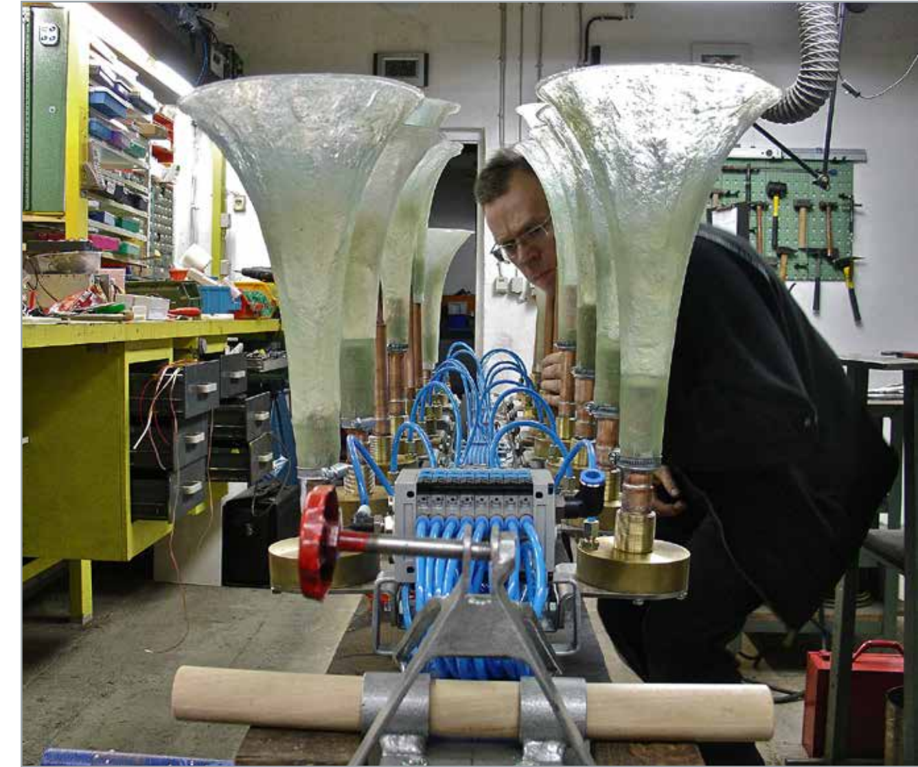
Assembly of a group of horns with synthetic resin bells
